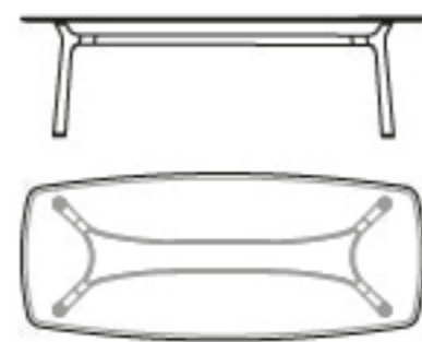
72611 Tavolo rettangolare inserto in marmo calacatta oro, cristallo grigio Rectangular table insert in calacatta gold marble, grey glass cm 260 x 108 x h 74 in 102 3/8 x 42 1/2 x h 29 1/8
