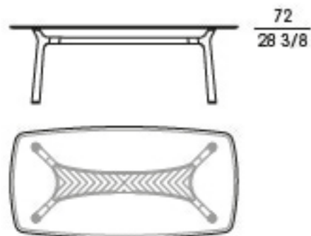
72600 Tavolo rettangolare inserto in frassino, cristallo grigio Rectangular table insert in ash wood, grey glass cm 220 x 108 x h 74 in 86 5/8 x 42 1/2 x h 29 1/8
