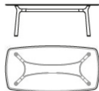
72610 Tavolo rettangolare inserto in marmo calacatta oro, cristallo grigio Rectangular table insert in calacatta gold marble, grey glass cm 220 x 108 x h 74 in 86 5/8 x 42 1/2 x h 29 1/8
